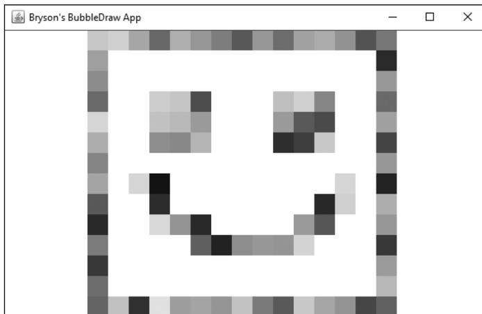
Figure 9-9: Drawing with rectangles instead of ovals creates a pixelated drawing effect.
