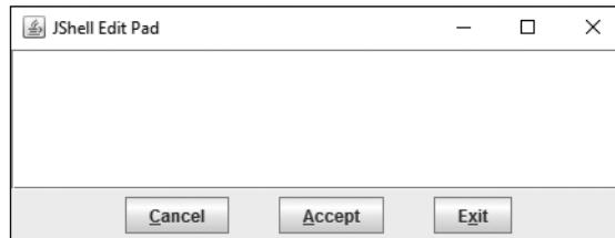
Figure 3-3: The JShell Edit Pad is a convenient editor for writing longer snippets of code.
