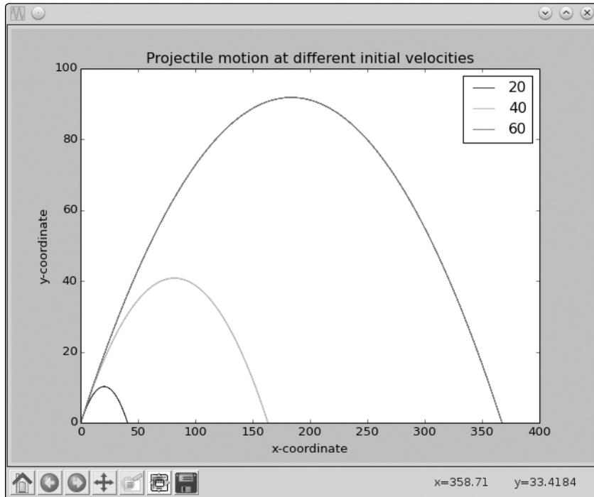
Figure 2-15: The trajectory of a ball thrown at a 60-degree angle, with a velocity of 20, 40, and 60 m/s
